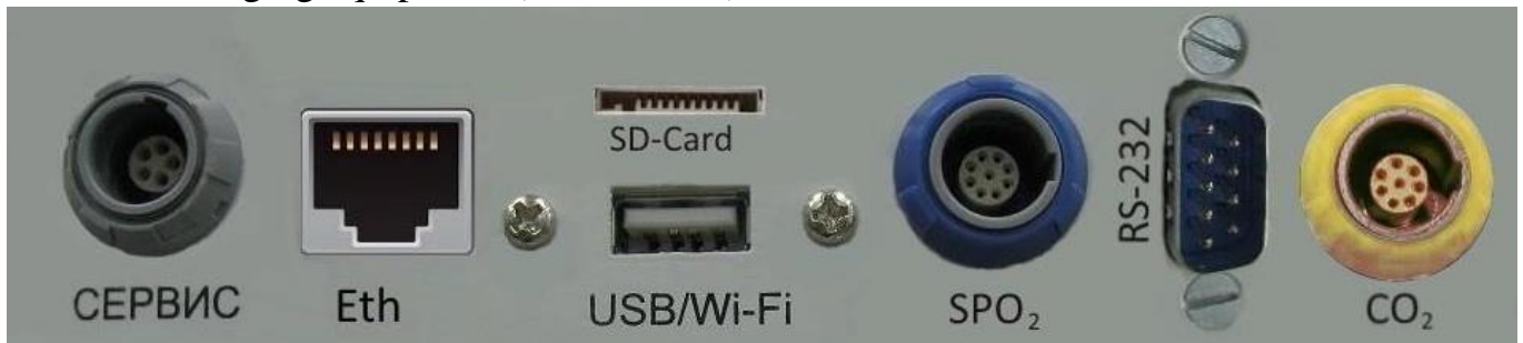
Picture 5.25- Connectors for connection of additional equipment
