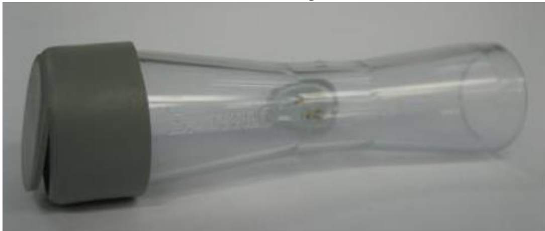
Picture 5.20- Placement of the check valve on the flow sensor
