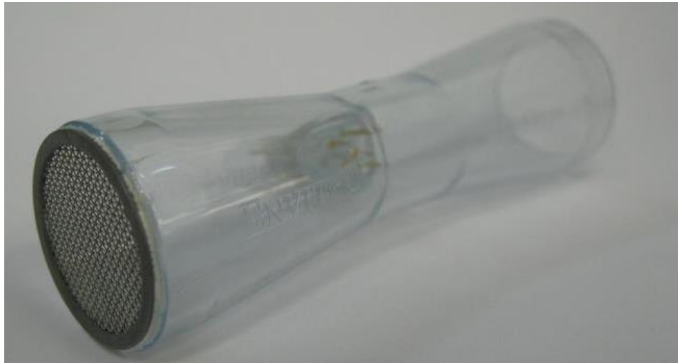
Picture 5.19- Placement of a grid on the flow sensor
