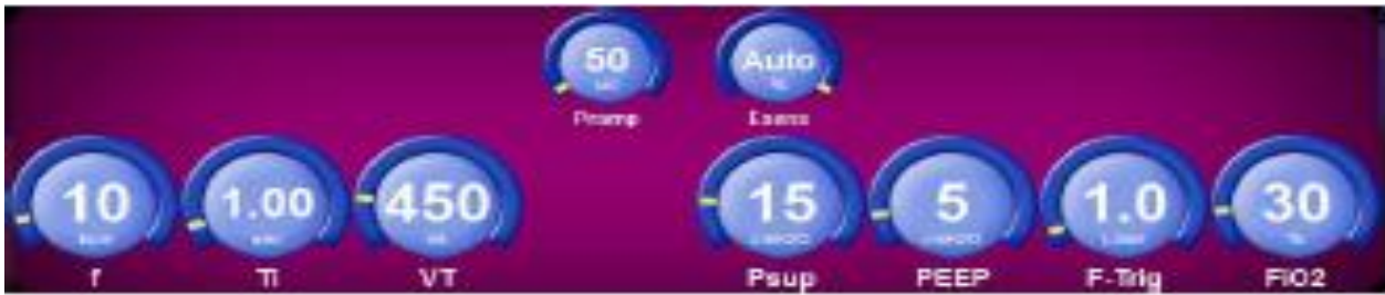
Picture 7.7 – Panel of the control additional parameters
