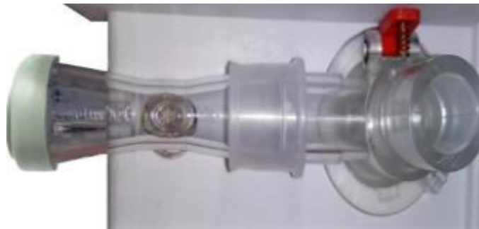
Picture 5.22- Location of flow sensor on the ventilator
