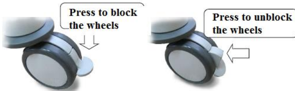
Picture 5.26-Control the ventilator blocking mechanism of the wheels
